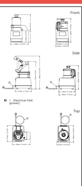
Electric Supply voltage: 220-240 V/1N ph/50 Hz Electrical power max.: 0.5 kW 0.5 kW **Total Watts:** Capacity: Performance (up to): Capacity: 2.6 litres Key Information: External dimensions, Width: 348 mm External dimensions, Depth: 328 mm External dimensions, Height: 527 mm **Shipping weight:** 21.1 kg Net weight (kg): 14.1 **Cold water paste:**
